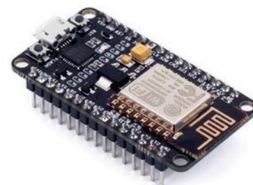
■ FIGURE 2. The $10 NodeMCU Amica R2 module containing the ESP8266-12.
